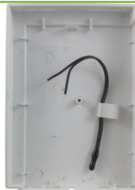
Figure 1-2: Inside the Allure EC-Sensor-T enclosure - temperature sensor (thermistor), approximately 4.75 inches (12 cm) of wire and a clip to hold thermistor/wire in place.
