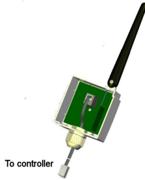
Figure 17: Location of the Wireless Receiver's telephone socket
