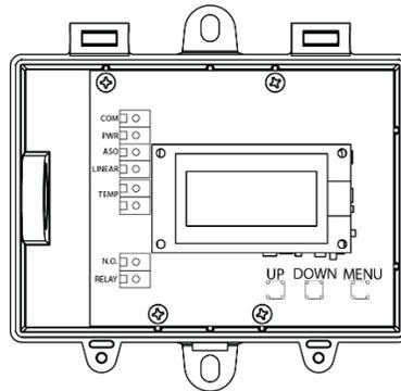
Figure 6: Connector layout.
