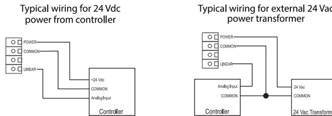
Figure 7: Typical AC or DC wiring
