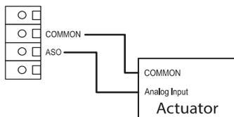
Figure 8: Direct connection to a damper actuator.
